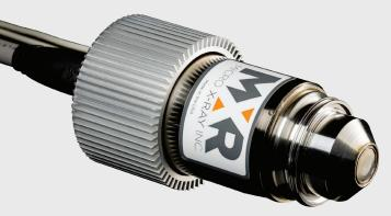
The LightBright is an end window X-ray tube designed for customers that require maximum flux, short FOD and a wide beam angle. The large heat sink directly coupled to the anode provides efficient heat transfer enabling continuous high current operation, and the optimized filament design provides full beam current down to 4kV without sacrificing tube life. The integrated Mammoflex® HV cable and LV cables allow for easy connection to a standard HV power supply.
