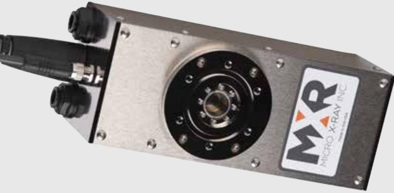
Our SeeRay series is designed with a diamond anode and direct anode water cooling which enables power densities up to 1.5W/ $\mu\text{m}$ , power up to 100W, and ultra-fast spot stabilization time. The SeeRay is fully radiation shielded, high voltage isolated, and includes both high voltage and low voltage cables.
